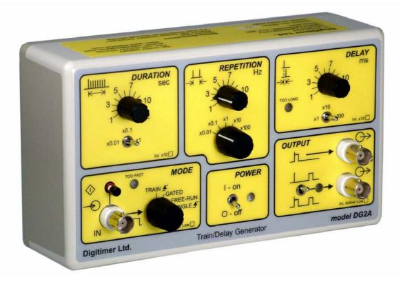
The DG2A is a compact, free-standing, battery powered instrument which can be used to generate trigger pulses required for repetitive stimulation. Also featuring DELAY controls, it is useful for determining nerve or axonal Effective Refractory Period (ERP) through the production of a delayed second pulse.
