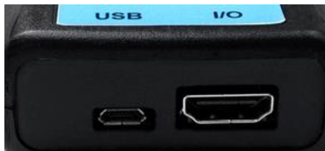
Right panel: Micro-USB port (left) for connecting Smart Center to computer and I/O port (right) for inputting digital signals
